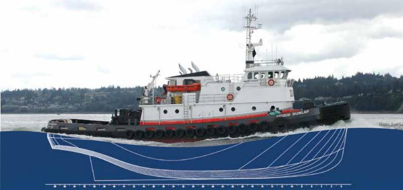
Our hull form development begins with your performance requirements and focuses on minimizing vessel motions as well as optimizing flow to propellers for maximum bollard pull. Our hull design approach extends to the entire propulsion system toward selecting the most appropriate application of direct drives, azimuthing drives, and open or nozzled propellers.
